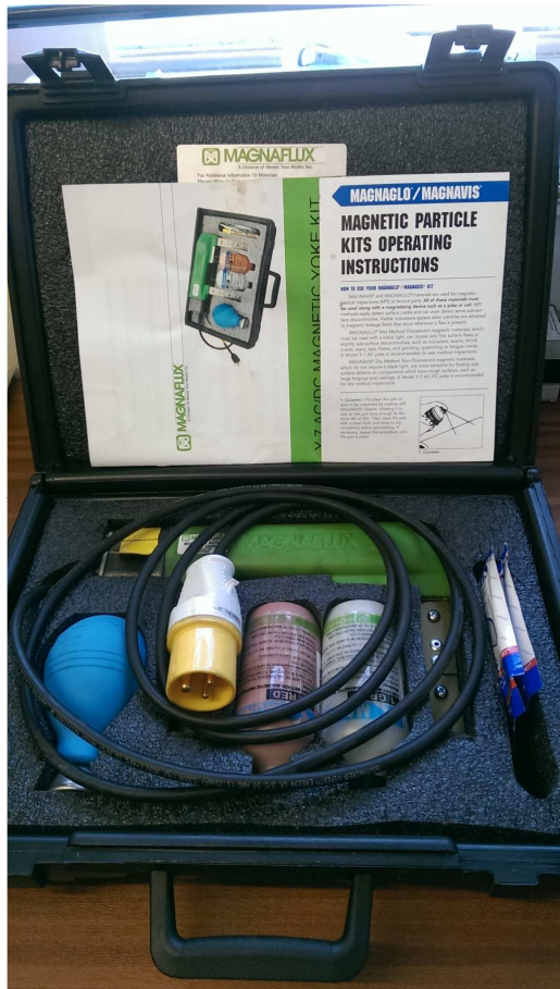
Y-7 AC/DC Magnetic yoke kit
